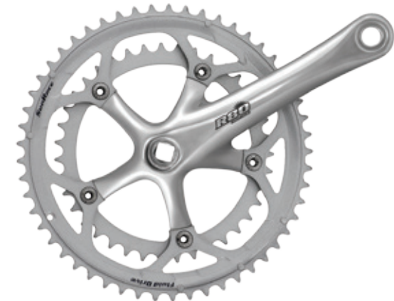
FCR810 53-39T FCR830 52-42T FCR87 52-42-30T · 8-Speed · 6061 Forged Alloy Crank · SCM435 Bolts & Nuts
