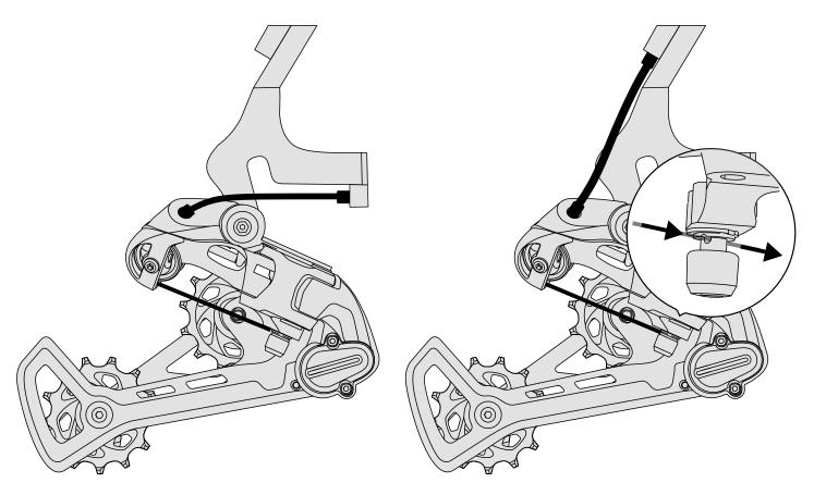
4. Using the high and low adjustment screw fix the high and low limits.
