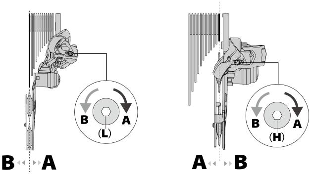
5. Set the rear derailleur to the largest sprocket and adjust the end adjuster screw with a 2mm Allen key so that the clearance between the tip of the guide pulley and the tip of the largest sprocket is within the range.
