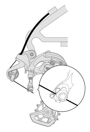
4. Adjust the high and low adjustment screw for setting the high and low limit.
