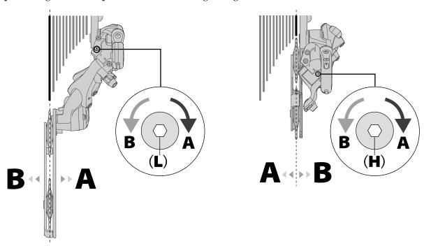
5. Set the rear derailleur on the largest sprocket adjust the end adjust screw with a 2mm Allen key so that the clearance between the tip of the guide pulley and the tip of the largest sprocket is within the range.
